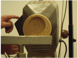
The third project was more advanced, an off-centre bowl. The blank was drilled in two places to take a screw chuck, one in the centre and one off-set. After turning the under-side centrally, it was mounted offcentre to cut a dovetailed recess, on which it was held to turn the bowl, which was, of course, off-centre. Seems like an easy way to do it. Above we see the bowl part finished.
